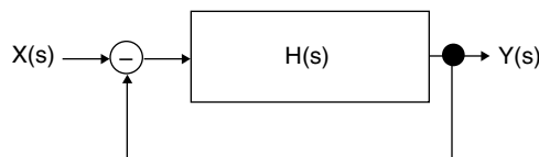
FIGURE 7.2 A linear servomechanism. X(S) is the representation of the input signal. Y(S) is the representation of the output signal. H(S) is the representation of the “transfer function,” a mathematical expression that completely characterizes the linear servomechanism. The “-” sign in the circle indicates negative feedback; a replica of the output signal is coupled in parallel but out of phase with the input signal.
