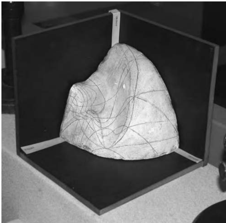
FIGURE 9.1 (See color insert following page 150.) Plaster model of the equilibrium states of water constructed by James Clerk Maxwell and sent as a present to Josiah Willard Gibbs. (©The Cavendish Laboratory, University of Cambridge. Reproduced with permission.)
